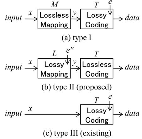
Fig.3 ‘Lossy’ encoding for sparse histogram images.
