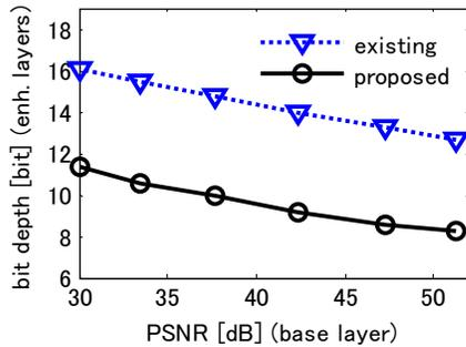
Fig.8 Bit depth of the enhancement layer (color).
