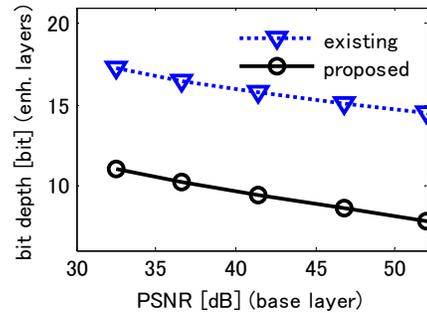
Fig.10 Bit depth of the enhancement layer (Luminance).
