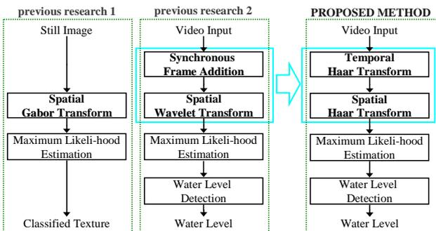
Figure 4 Unification of the temporal and spatial filtering.
