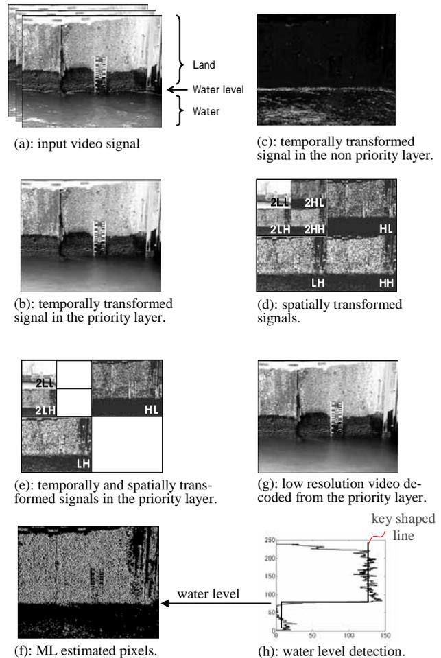
Figure 5 Signal processing example.
