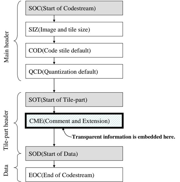
Fig.5: Bit stream composition of the system.
