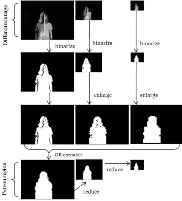
Fig.4: Moving object extraction using wavelet transform.
