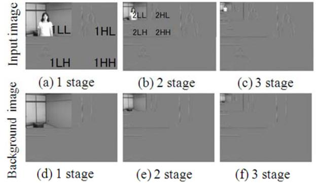
**Fig.2:** Subband decomposition using wavelet transform.
