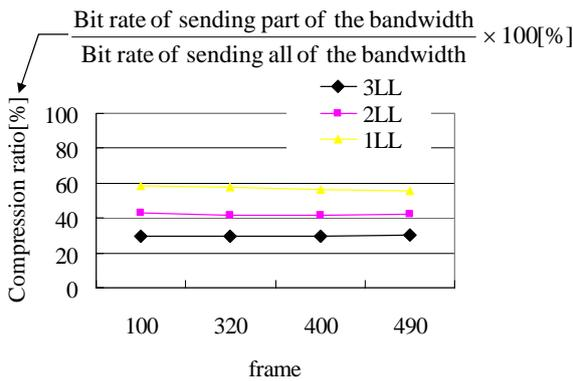
Fig.12: Compression ratios for sending part of the bandwidth and for sending all of the bandwidth.
