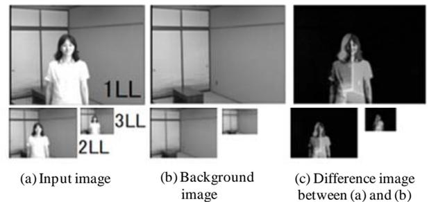
**Fig.3:** Image subtraction between the current input image and the background image.
