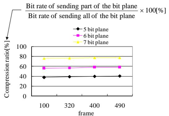
**Fig.10: Compression ratios for sending part of the bit plane and for sending the entire bit plane.**
