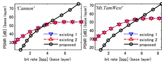
Fig.5 Rate distortion curves in the base layer.
