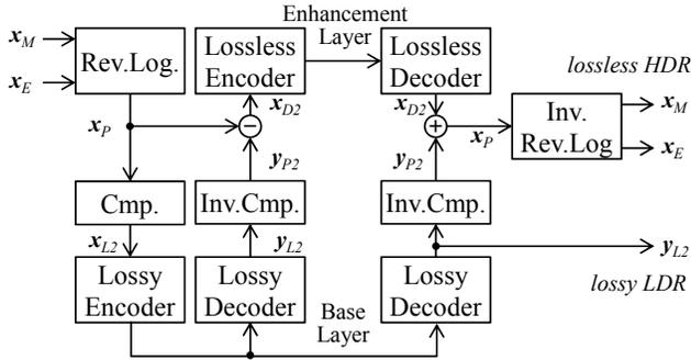
Fig.2 Existing method 2. Reversible logarithmic mapping (Rev.Log.) reduces bit depth of  $x_P$ . Compensation (Cmp.) produces a tone mapped LDR image  $x_{L2}$ . However its inverse magnifies coding noise.
