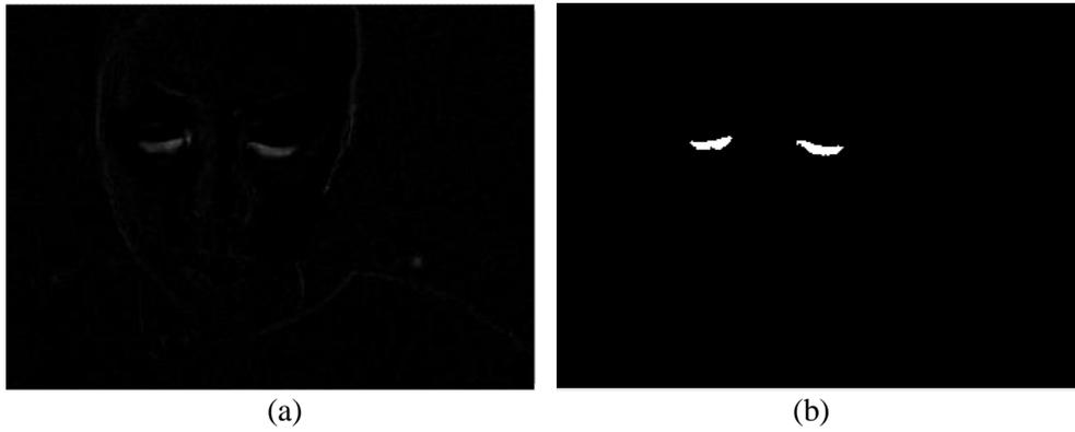
FIGURE 3. (a) Image subtraction of previous and current frames, (b) Thresholded image of the subtracted image.
