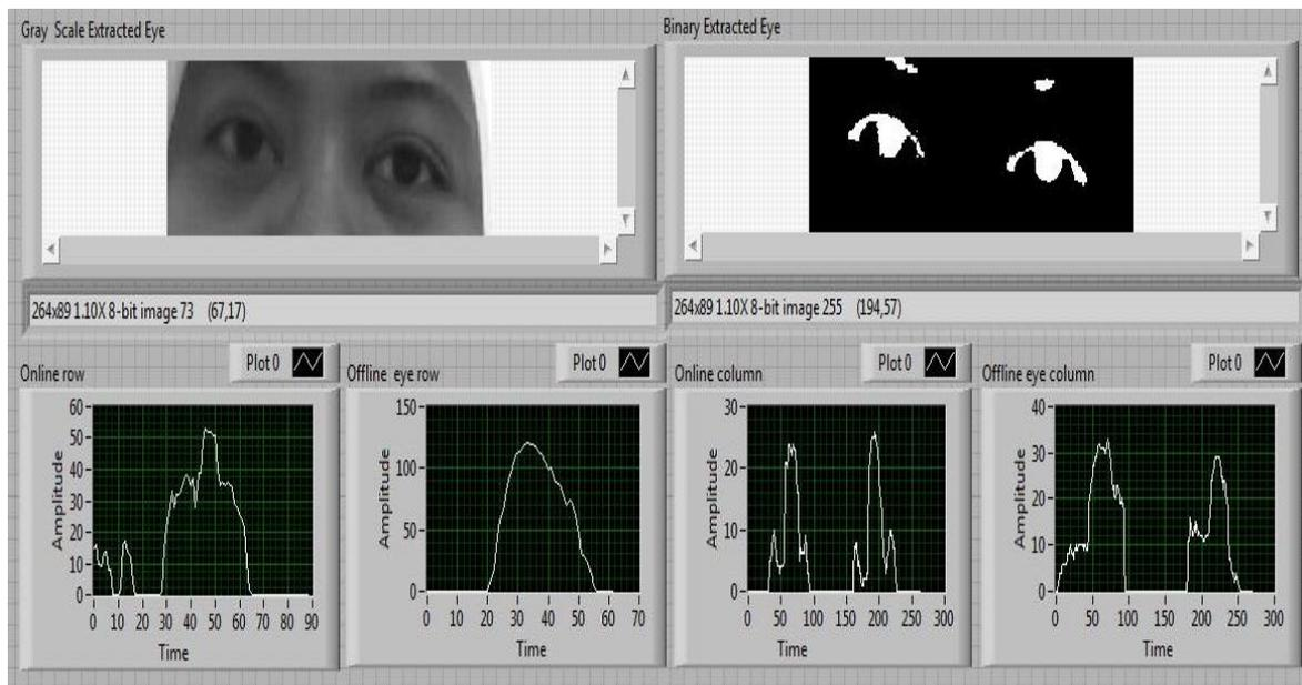
FIGURE 7. Adaptive region of interest with the extracted image in gray scale, binarization of image, offline arrays and online arrays.
