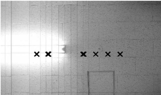
Fig.2 Ceiling map generated from an upward camera of a robot moving on a non-flat floor.
