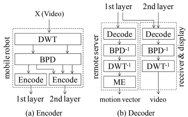
Fig.6 Encoder and decoder of the existing FLC in [8]. ME: motion estimation, BPD: bit plane decomposition, DWT: discrete wavelet transform.
