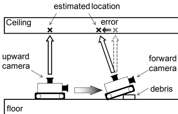
Fig.4 Location estimated from an upward camera of a robot contains error due to debris on the floor.
