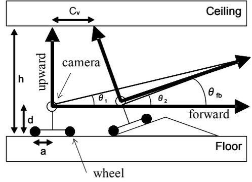
Fig.7 Analysis model for compensation of motion information of upward video by that of forward video.
