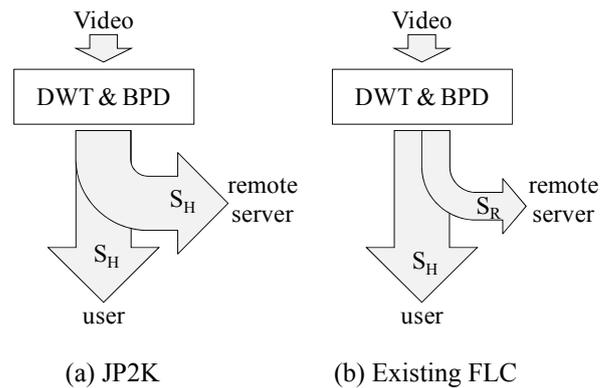
Fig.5 The existing FLC in [8] transmits the minimum data to a remote server necessary for motion estimation.
