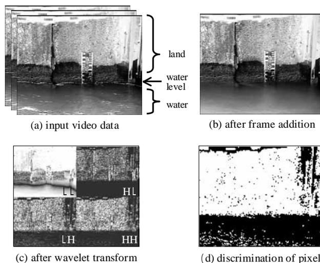
Figure 1 Each pixel is classified into water or land with wavelet transform in JP2K and ML estimation. Boundary of the two regions is detected as the water level.
