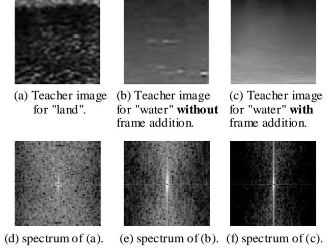
Figure 2 Teacher images and their spectra. The frame addition procedure reduces signal components in high frequency in the running "water" region.
