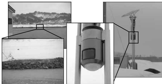
Figure 9 A video sensor installed in Niigata for 24 hours-a-day monitoring of the river and its video signal output.
