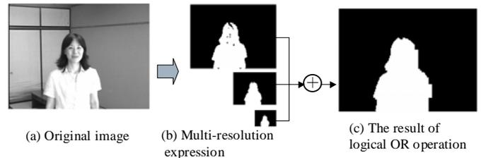
**Fig.4:** Moving Object extraction results. Undesired holes in the object region are reduced by proposed method.
