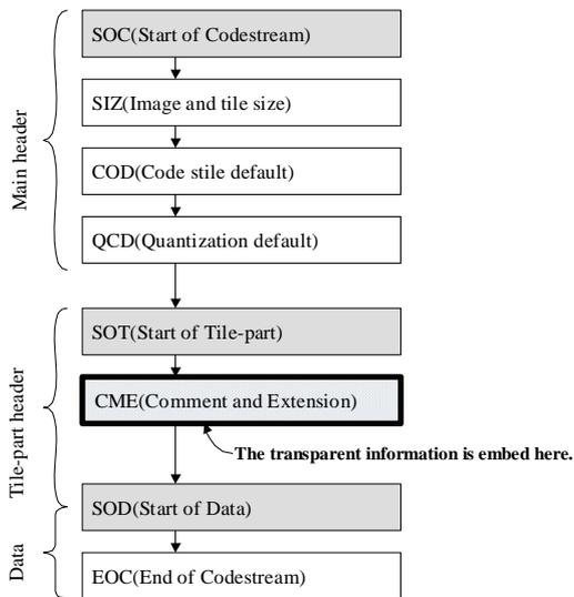
Fig.5: The bit stream composition of the system.
