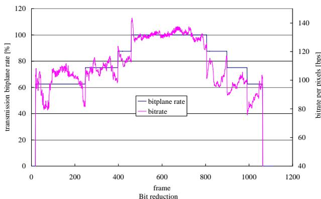
Fig.8: Bit rate for sending only the upper bit plane(semi-transparent image)
