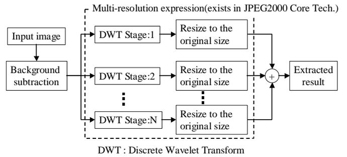
**Fig.3:** Moving person extraction by using multi-resolution expression(proposed method).
