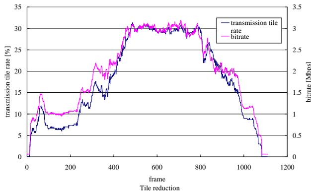
Fig.7: Bit rate for sending only person's tile
