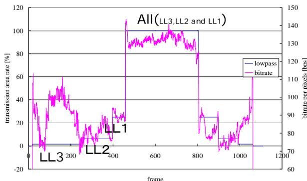
Fig.9: Bit rate for sending only a part of bandwidth(low pass image)
